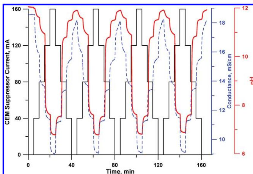
**Figure 3.** Step gradient response. Four cycles are shown for a  $\text{Na}_3\text{PO}_4$  feed CEM suppressor system with an influent flow of 1 mL/min. Current steps are 0 → 40 → 80 → 120 → 160 → 120 → 80 → 40 → 0 mA (solid black). pH response is in the thicker line (solid red), and conductivity response is the dashed line (blue).
