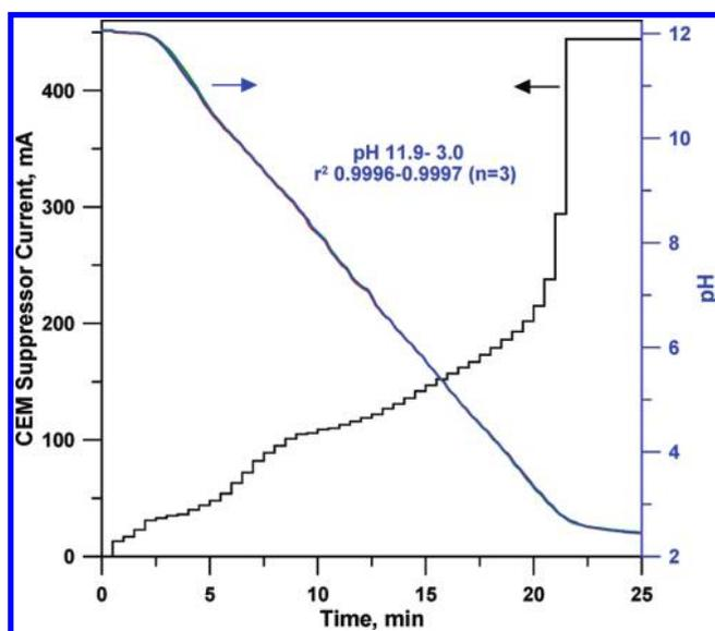
**Figure 6.** Three repeated 25 min linear pH gradient runs overlaid (right ordinate); the current program uses the left ordinate.
