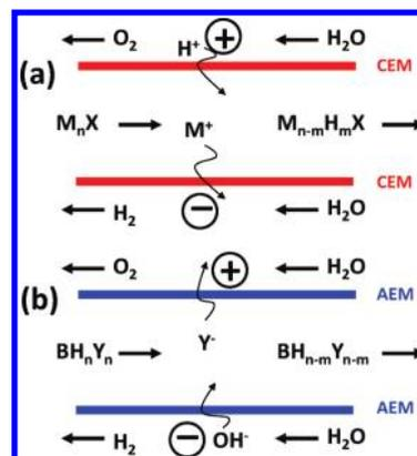
**Figure 1.** EBG scheme with (a) an anion suppressor (a dual CEM device) with the strong base salt of a multiprotic acid as the feed solution and (b) a cation suppressor (a dual AEM device) with the strong acid salt of a multiprotic base as the feed solution. The drive current controls how much of the strong base cations in panel a and the strong acid anions in panel b are respectively removed from the system to attain the desired pH.
