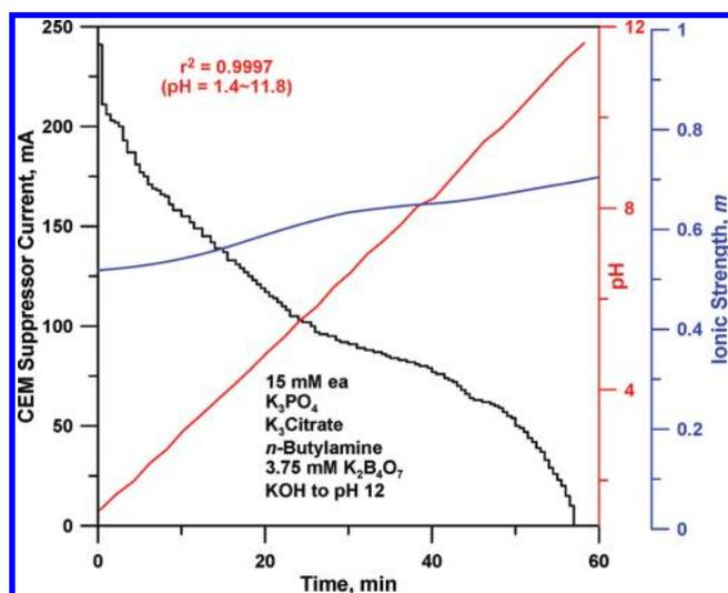
**Figure 7.** A four-component buffering mixture with an increasing linear pH gradient in the presence of large amounts of NaCl. Without the presence of the salt, the ionic strength will change by more than an order of magnitude (see Figure 5a).
