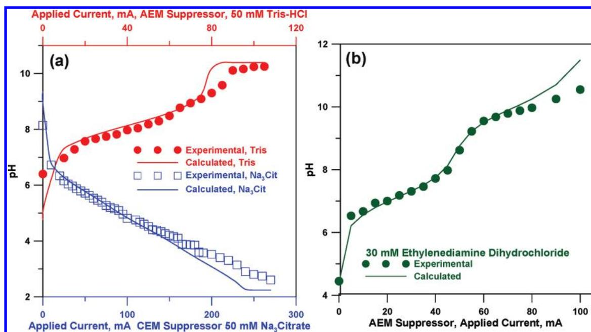
**Figure 4.** pH as a function of drive current for (a) 50 mM trisodium citrate as the feed solution (ASRS Ultra II, 4 mm) and 50 mM Tris-HCl (CSRS Ultra, 4 mm), and (b) 30 mM ethylenediamine dihydrochloride (CSRS Ultra, 4 mm), all at 1.00 mL/min. Solid lines represent computed pH values; see text.
