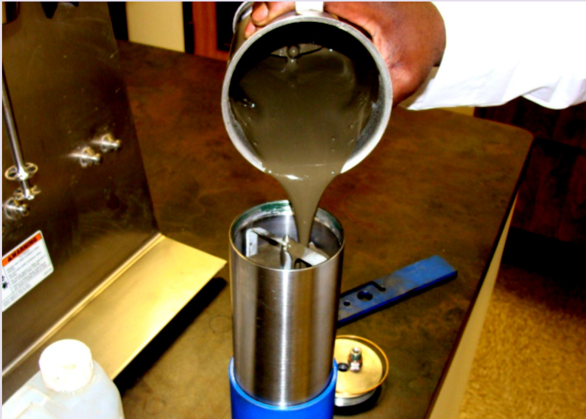
FIGURE 1. The picture reflects the reduction in apparent viscosity and the ease of pouring of the cement slurry after treatment with CD-U7 .
